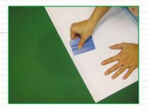
4. Slide the graphic into the profile and secure with a piece of tape at the back.
