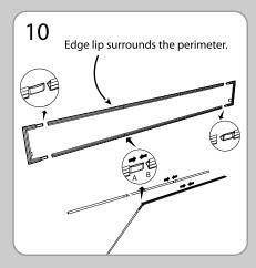
Assemble the upper and lower straight sections by inserting A side (with metal spring) into B side, as shown in detail illustration above. Insert the U-shaped end pieces into the ends of the assembled straight sections.
