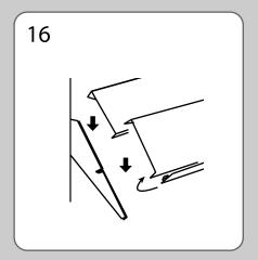
Snap the literature strip onto the front edge of the shelf after shelves are installed.
