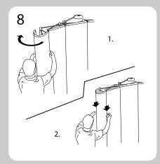
1. Lift end panel and guide front notch of plastic plate over front peg. Hook the other side on the panel peg at the back of the frame.
