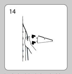
Insert bracket tabs into the slots and push down into place.
