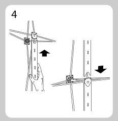
Begin at the bottom center module and attach channel bars by sliding up onto the upper hub. Line up the bottom of the channel bar over the lower hub and slide down to secure. Leave the top front row open for top channel bars.
