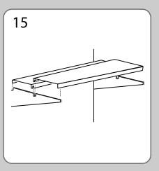
Place the second bracket level with the first. Attach each shelf with the notches facing the back. Secure each shelf by making sure it is pressed down into the slots in the brackets.
