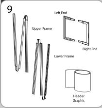
To assemble the Backlit Header: Unpack and identify frame parts shown above.
