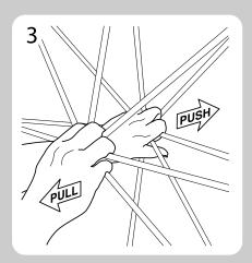
To close the frame: While tilting the frame towards you, push and pull from the middle of the frame while grasping the hubs as shown. Once the frame starts to collapse, move hands away from the hubs to avoid pinching. Do not pull tubing alone.
