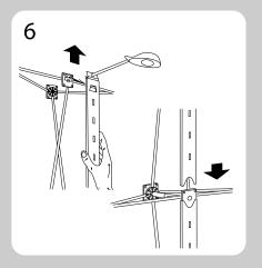
Mount top channel bars (with lights attached) to frame by aligning hole in channel bar over panel pegs on top hub and sliding up. Once top of channel bar is in place, slide channel bar down onto bottom hub to secure.
