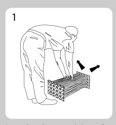
Remove frame from case and place on floor. Place frame with the yellow dots on the bottom facing you. Grasp upper ends of frame and pull up and outwards. Continue pulling up and outward until the frame is fully expanded.
