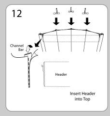
Lift the completed header assembly and hang it by inserting the brackets into the top of the channel bars. Hang lights by inserting the light bracket into the top of the channel bars.
