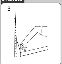
From the bottom, pull the panel away from the frame to expose the slots in the channel bar
